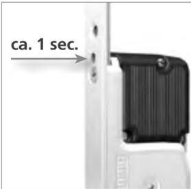
1. Carefully press the programming button on the Smart radio module for approx. 1 second.
