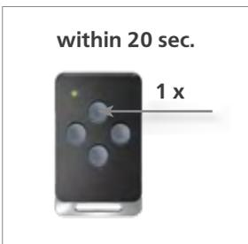
3. Press the transmit button on the user SmartKey you want to delete, within 20 seconds once.
