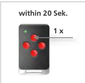
2. Press the tuning in and opening button on your master SmartKey within 20 seconds once.
