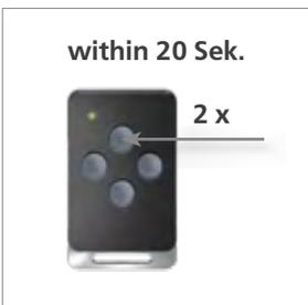
3. Press the transmit button on the SmartKey to be tuned in within 20 seconds, twice.
